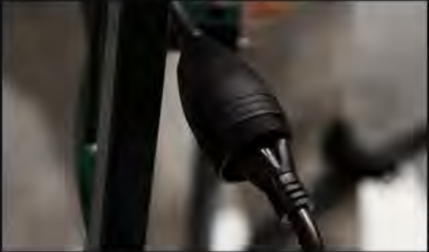
Booted main harness female receptacles to further shield moisture away from plugs.
